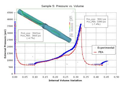
Caption: Collapse analysis of pressurized pipe can be performed with ADINA software.
