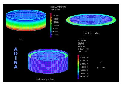
Caption: Sloshing of an oil tank with the base subjected to horizontal ground motion with ADINA software.
