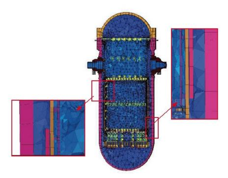
Caption: Simulation of a pipe break in a nuclear reactor using ADINA technology.
